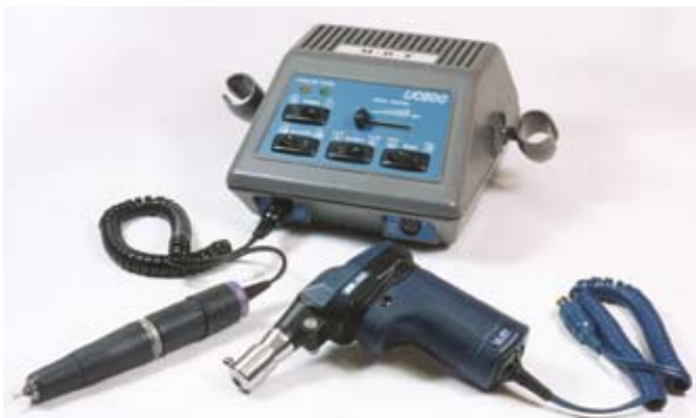
Ultrasonic systems consist of an electronic power module (110 or 220 volt) and a slender, electric cord that powers a very lightweight ultrasonic handpiece.
